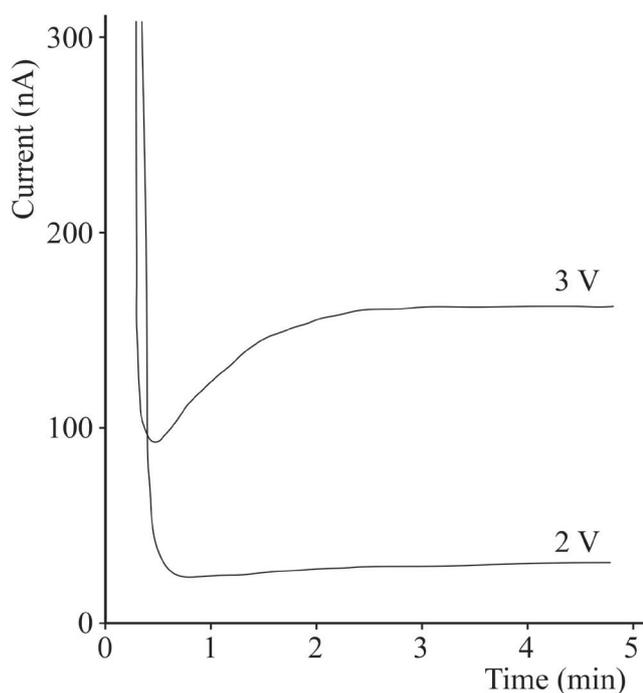
Figure 3. Current response during the electropolymerization of poly(oxyphenylene) on the carbon surface of the microelectrodes at two different holding potentials. The dip in the response at 3 V is due to a higher steady-state current eventually reached and may reflect uneven polymer formation.
