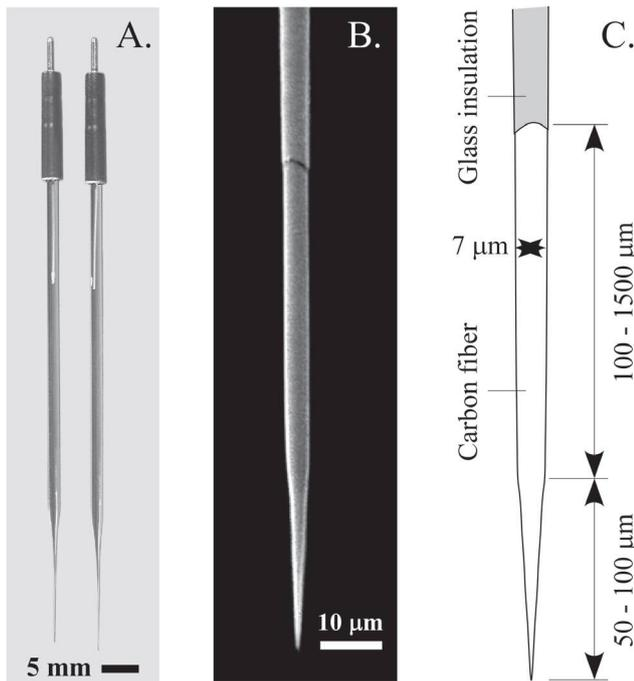
Figure 2. Macroscopic (A) and scanning electron microscopic (B) view of single-barrel carbon fiber microelectrodes made for submicron-scale electrophysiological, electrochemical or biosensor applications. Section of the carbon fiber protruding from the glass insulation (B,C) allows shaping of submicrometer tips. The exposed carbon surface can be modified chemically and is to be insulated by electropolymerization. Ultrasmall electroactive area can be formed on the very tip.
